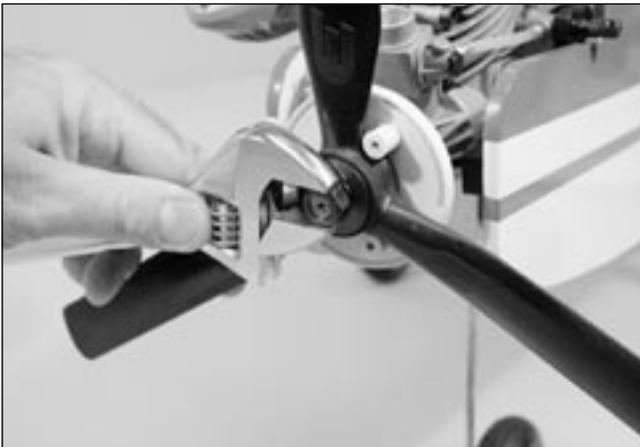
**Warning:** The propeller must be securely tightened before attempting to run the Evolution engine. Be sure to check the propeller before each flying session.
